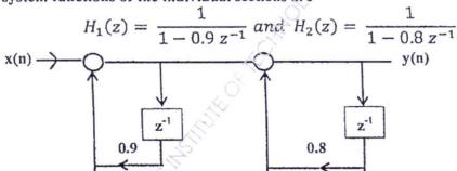
Draw product quantisation noise model of the system and determine the overall output noise power
